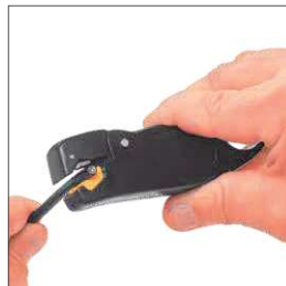
Inserting a coax cable
