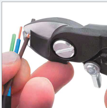
Stripping NYM/NM-B wire (1.5mm 2 – 2.5mm 2 )
