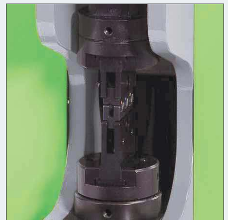
Model CM 25-6 – crimping machine with reduced stroke, without guards
