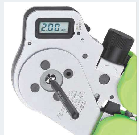
Pliers can be calibrated by the user
