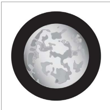
POF cable cut with conventional tool – time-consuming polishing is needed
