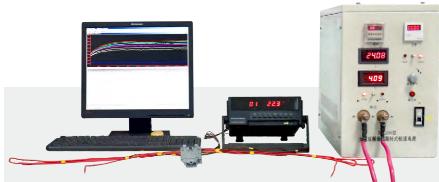
Din Rail Terminal Blocks Temperature-rise Test
