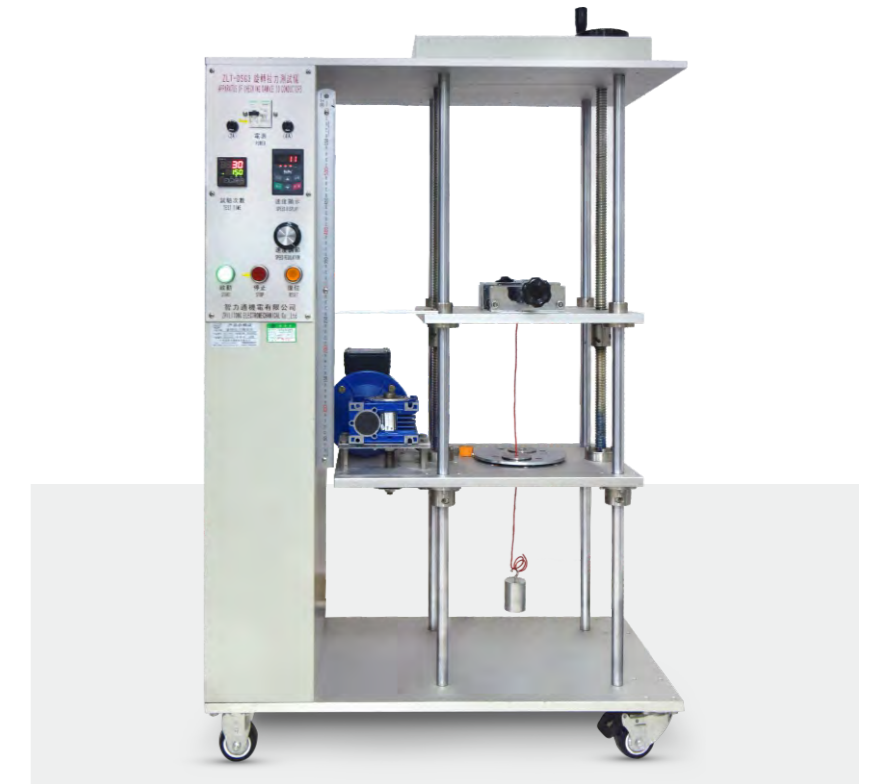
Din Rail Terminal Blocks Rotational Pull Test
