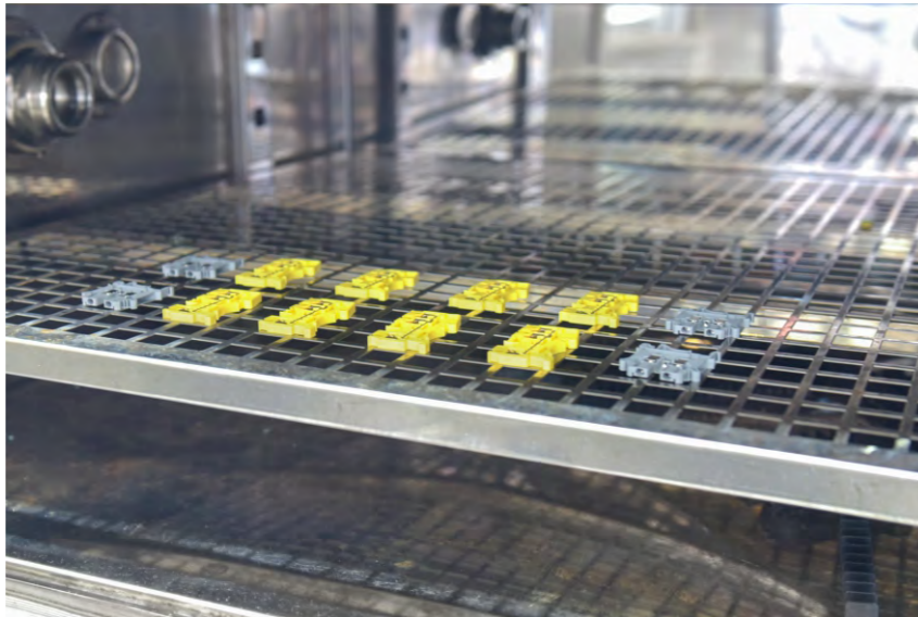
Din Rail Terminal Blocks Temperature Cycling Test
